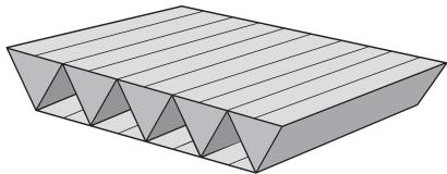
Cordion panels can be flat, curved, or a combination of both. They can fold in a straight line, or radially like a fan. Cordion panels can be supported on their edges, they can be supported internally, they can be held in tension by cables, and they can be designed to self-extend.
